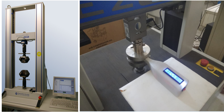
Fig. 9. Calibration Setup on UTM Machine
