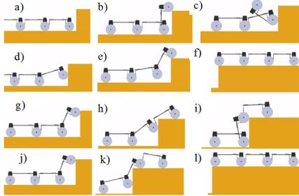
Fig. 6. Step climbing ability of the 3-module robot: a)-c) Case-1: the passive robot tips over while climbing a height of 14 cm; d)-f) Case-2: it successfully climbs the step of 14 cm using a compliant joint at  $J_1$ ; Case-3: g)-i) the robot with a compliant joint at  $J_1$  manages to climb a height of 16 cm but is unable to pull the remaining links; Case-4: j)-l) it is able to fully climb a height of 16 cm using compliant joints at  $J_1$  and  $J_2$
