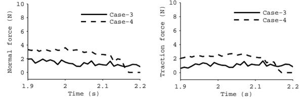
Fig. 8. Utility of spring at  $J_2$  while climbing a step of 16cm: Plots showing the variation Normal and Traction forces at wheel 2 with spring (Case-4) and without spring(Case-3) at  $J_2$ .
