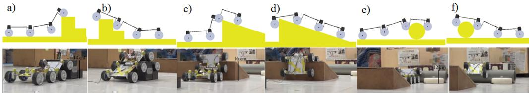
Fig. 10. Demonstrating the climbing ability of the 3-module robot in simulation (top row) and experiment (bottom row): In a)-b), the obstacle is a rectangular block of 14 cm height; In c)-d), it is wooden ramp of maximum height 16 cm; Finally, in e)-f), the obstacle is a cylindrical pipe of 12 cm diameter
