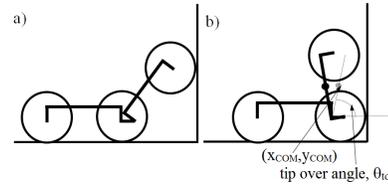
Fig. 3. Climbing behavior of the passive robot
